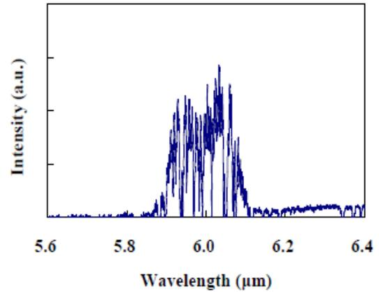
Fig.2. Lasing spectrum of a 6  $\mu$  m FP-QCL.
