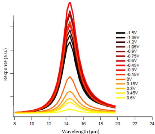
*Result of the modeling of 15 $\mu\text{m}$  VLWIR QCD: on the left are presented the current and noise modeling and measurement and on the right the response modeling*
