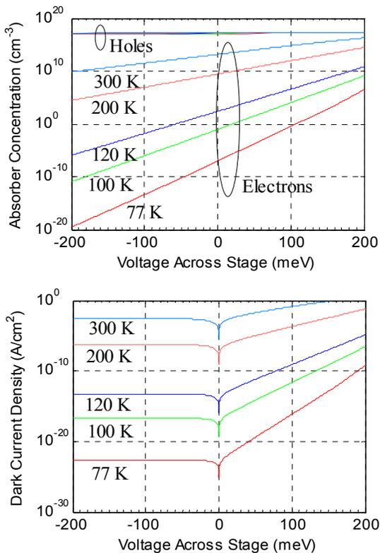
**Figure 1:** Voltage and temperature behavior for (a) carrier concentration of minority electrons and majority holes in the absorber and (b) generation-recombination current density.
