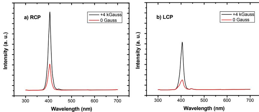
**Figure 2:** Right (RCP) and left (LCP) circularly polarized EL from Ga<sub>1-x</sub>Gd<sub>x</sub>N-based spin LED (plotted on same scale). Both right and left circularly polarized light are significantly in-creased by a 4 kGauss applied field.
