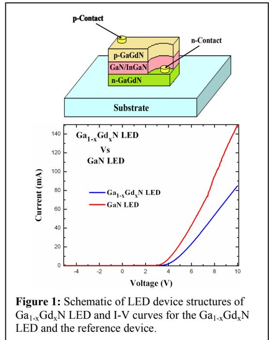
**Figure 1:** Schematic of LED device structures of Ga<sub>1-x</sub>Gd<sub>x</sub>N LED and I-V curves for the Ga<sub>1-x</sub>Gd<sub>x</sub>N LED and the reference device.
