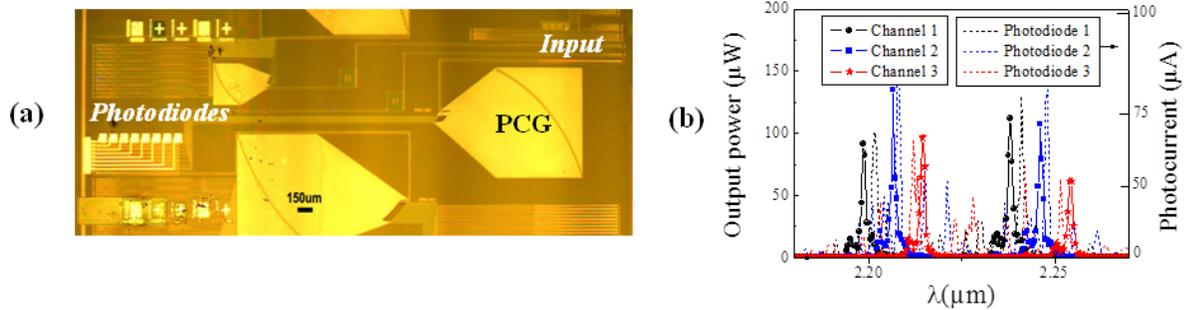
**Figure 1:** (a) Top view of a PCG spectrometer with integrated photodiodes processed at the outputs; (b) Comparison of the detected signal with and without photodiodes
