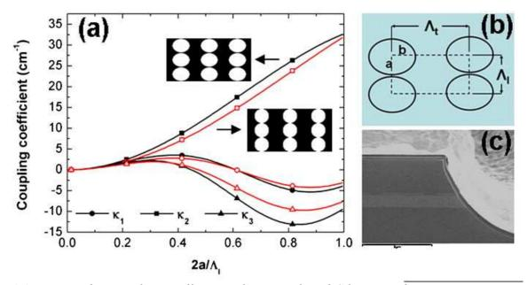
(a)  $\kappa_1$ ,  $\kappa_2$ , and  $\kappa_3$  coupling coefficients of rectangular PhC lattice with an aspect ratio of 2 with elliptical and circular features. (b) Depiction of the rectangular lattice dimensions with elliptical holes. (c) The cross section view of a cleaved facet and buried gratings on the finalized device.
