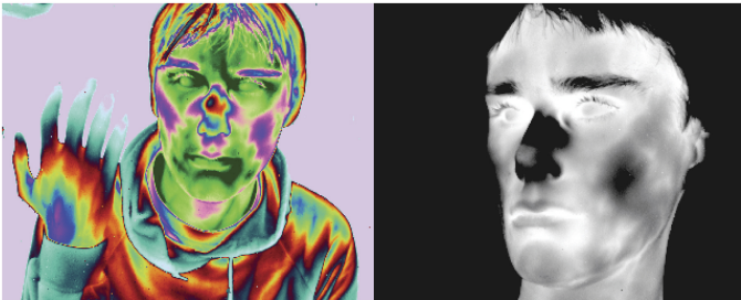
Figure 3. (Left) Images taken with a 3–5 \mu\text{m} IR camera based on type-II superlattices. (Right) Images from an 8–10 \mu\text{m} camera.
