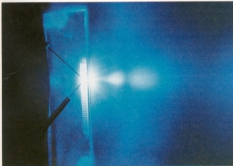
BLUE LIGHT streams from the edge of a GaN-based laser diode in the laboratory of Shuji Nakamura and his group at Nichia Chemical Industries in Tokushima, Japan. The light is made visible by its scattering off smoke particles, and the fluctuations in intensity of the light reflect the fluctuations in the density of smoke. Two needle-like electrodes are applied to the electrically pumped diode.
